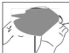
ENCAJE LA BOCA DE EN EL TECHO USANDO LAS GARRAS.
