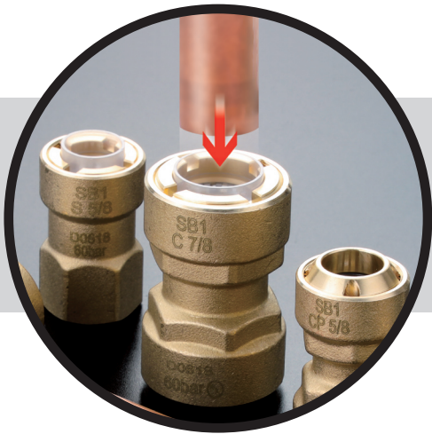
Quick Push Connector to Refrigerant Line
