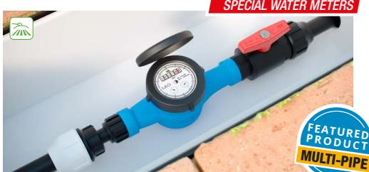
In the image we can see the installation of a water meter with the cut-off wrench, in which we can see the use of a connection with a free nut, which provides a point of dismantling for maintenance work, without having to completely disassemble the set.
