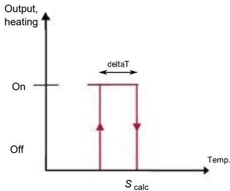
*Figure 2-2 Heating function*
