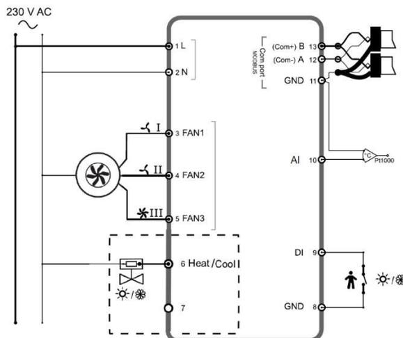
Figure 4-1 2-pipe wiring (standard)
