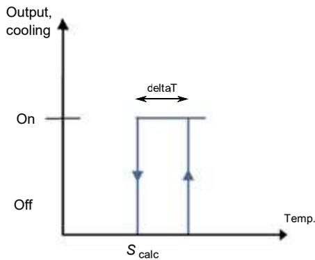
*Figure 2-3 Cooling function*
