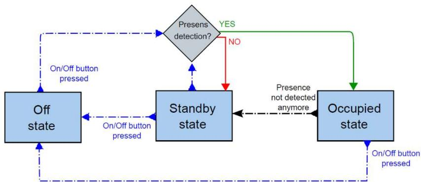
Figure 2-11 Changing controller states (no remote control)
