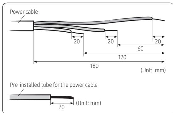
3 Insert the core wires of the existin and extending power cables into the connection sleeve.
