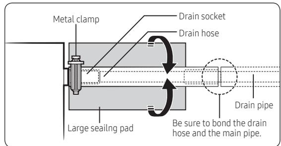
2 Tighten the metal clamp as shown in the figure.
