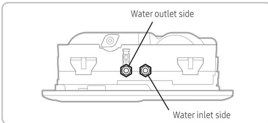
Be sure to check the water inlet and outlet locations.
